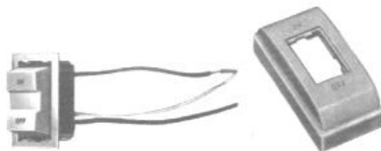
**Fig. 18-5** The type of switch used in remote-control wiring is shown above. The same kind of switch is used at every location. It is equivalent to two push buttons. Use as many switches as you wish to control one outlet (or several outlets if you wish). (General Electric Co.)
