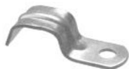
Fig. 8-16 Entrance cable must be anchored to the building every 30 inches. Use straps of the type shown. (The Hallex Company)
