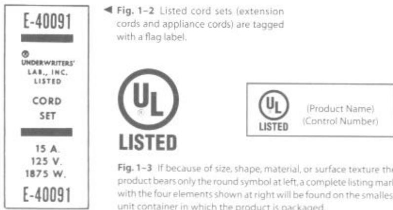
designed. Electrical inspectors will turn down listed merchandise if improperly used. For example, the inspector will refuse to accept listed armored cable used in a barn if the barn is a corrosive location, because armored cable is for use only in permanently dry locations. Listed lamp cord will be turned down if used for permanent wiring because such cord is listed only for use on portable equipment.
